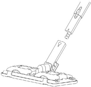
Floor brush nozzle to the end of extension tube. Ensure that nozzle clicks into place on assembly. The floor brush is ideal for cleaning washable wall and floor coverings. It may be used with or without the towel. Pressure on the inner side of the holder, open the clips to hold the towel.
